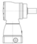
Mounting position B5/V3 (output shaft horizontal, motor shaft upwards)
