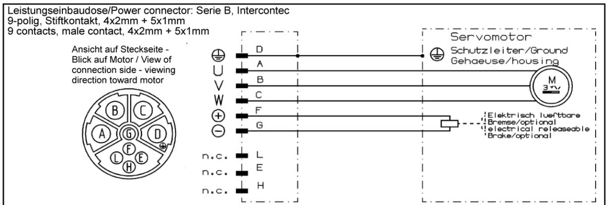
**Option “E” and “V” with 320 V intermediate voltage —signal (pin assignment 5)**
