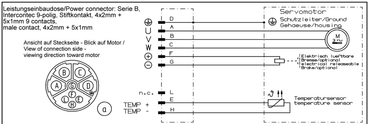
Design with resolver, EnDat- and Hiperface encoder —output size 1.5 (pin assignment 4)
