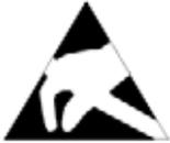
Component sensitive to electrostatic discharge
