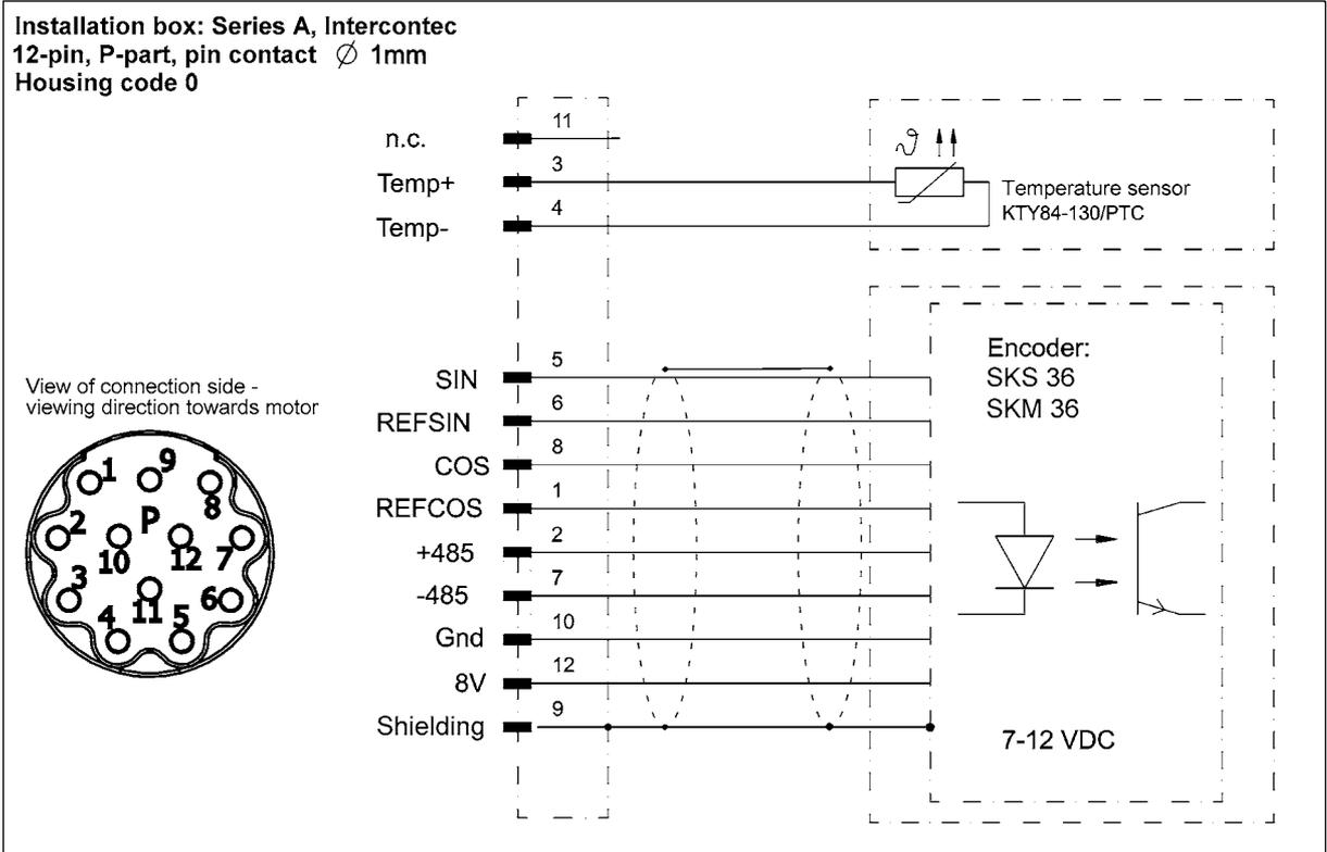
Option “S” and “M” —signal (pin assignment 1)
