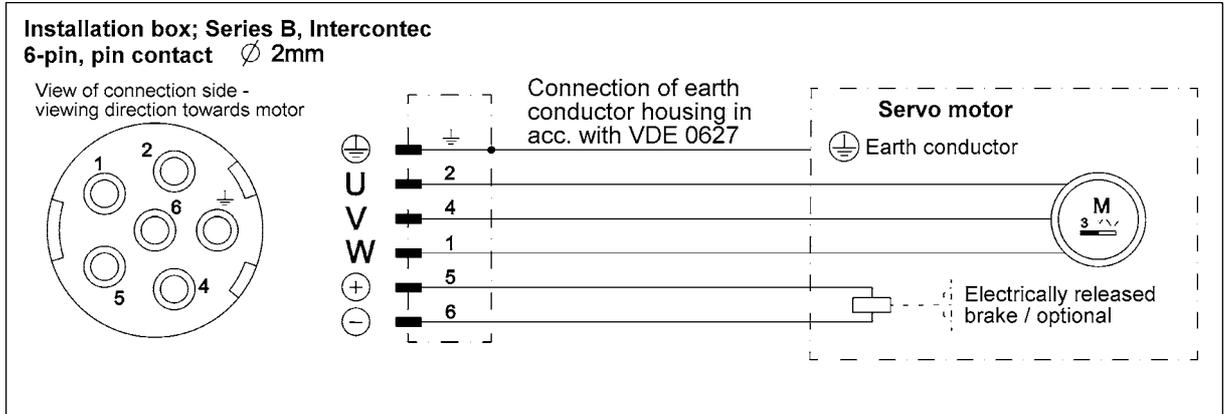
Design with resolver and optical encoder —output size 1.5 (pin assignment 1)
