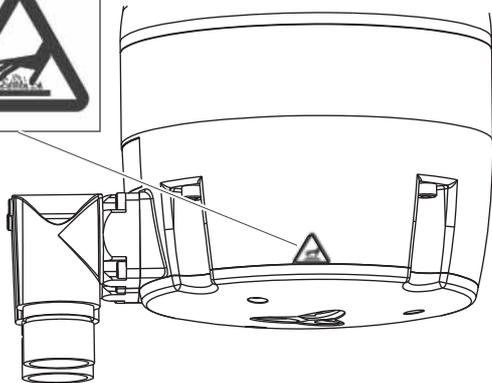
There is a safety sign on the servo actuator housing that warns against hot surfaces. This safety sign may **not** be removed.
