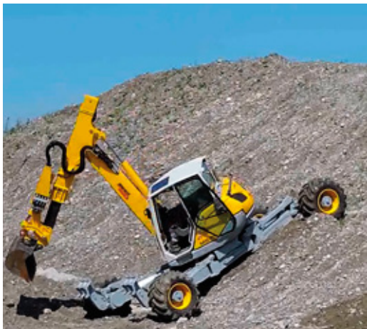
The excavator can be operated from a safe distance without any risk to life and limb.
