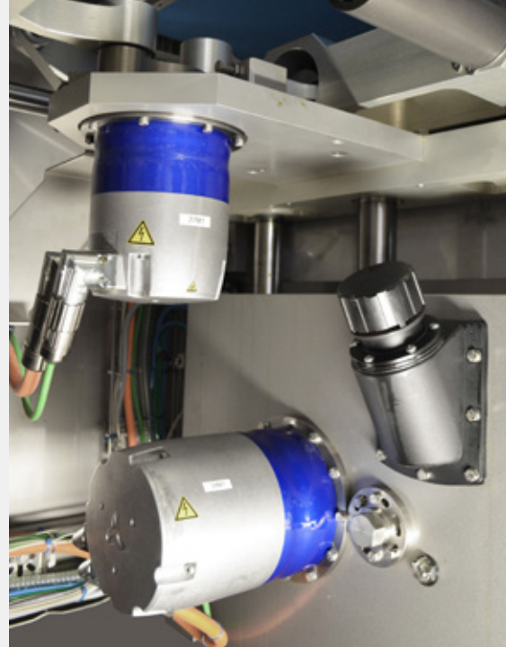
The TPM+ is installed in the jaw closer (top) and the jaw stroke (bottom)
